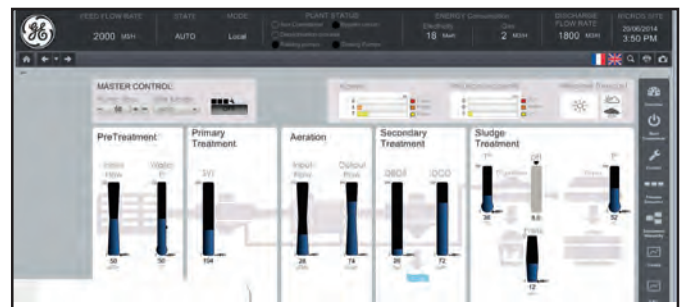
Operators and technicians can view workflows and develop a dynamic task list
